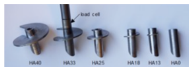
Examples of the scale models used; a shaft with a diameter of 10mm instrumented with 1:10 scale force sensors
