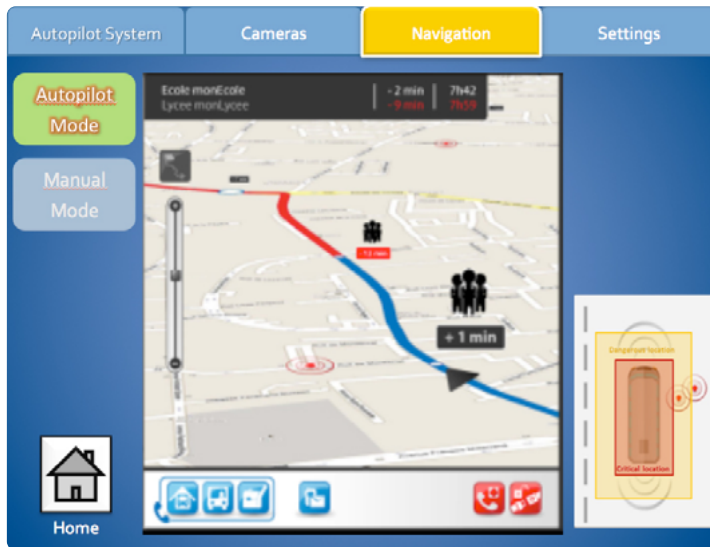
Proposed human-machine interface (HMI) specifications for buses with automatic docking Illustration © ADAS&ME
