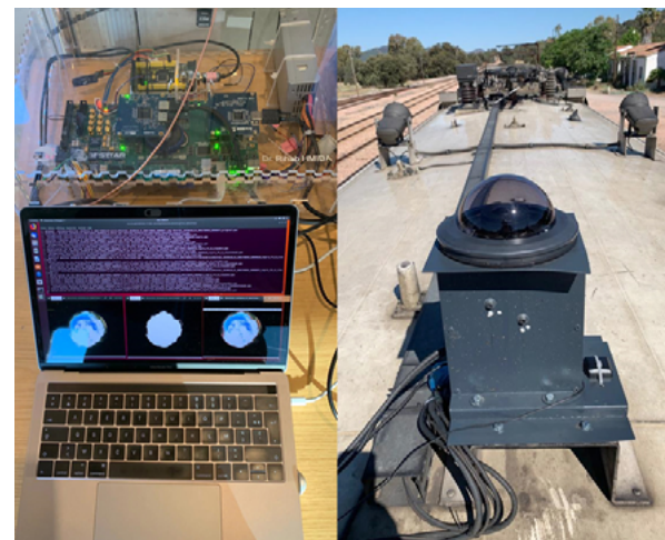
Equipment (PREDISSAT) developed by IFSTTAR and installed on a train for a campaign to detect the reception of indirect GNSS signals © Juliette Marais
