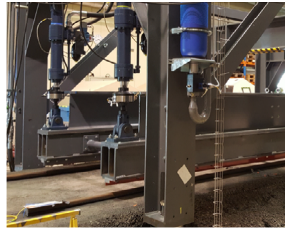
The SISYPHE platform used to test the railway structure in the REVES project
