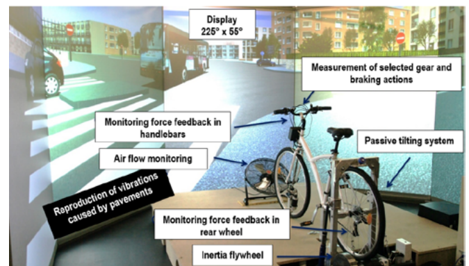
The bicycle simulator and its main functionalities © Stéphane Caro
