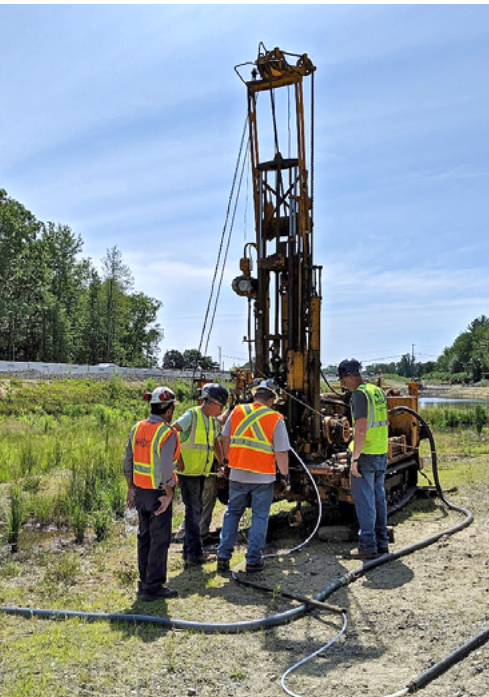
Perméafor tests developed by the University of New Hampshire (UNH) with the future Université Gustave Eiffel for the New Hampshire Department of Transport (NHDOT).
