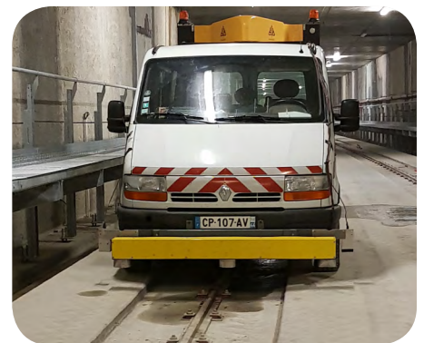
NEOVAL: Instrumented vehicle on a rolling test track
